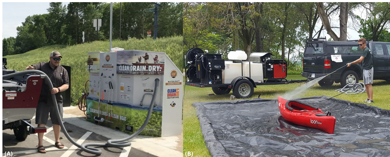
Figure 1. (A) A boater uses the vacuum tool of a waterless cleaning system (Credit: CD3 Systems). (B) A student uses the Michigan State University Mobile Boat Wash cleaning system, a high-pressure, hot water system. (Credit: J. Latimore).
