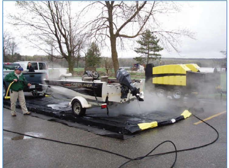
Portable decontamination station and water collection system (MN)
